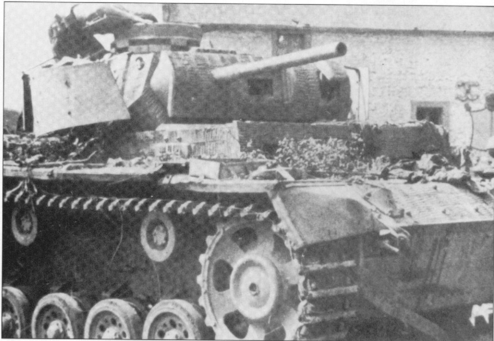
When the first German self-propelled artillery units were established, armored artillery observer's vehicles were developed using repaired Pzkw III MBTs. Extended radio equipment was added and the armament was deleted. This photo shows a derelict Pzbeobwg III Ausf. H. The dummy gun, which resembles a 50 mm gun, and the MG ball mount are visible. The Zimmerit was added by field workshops. (J. Mueller)
