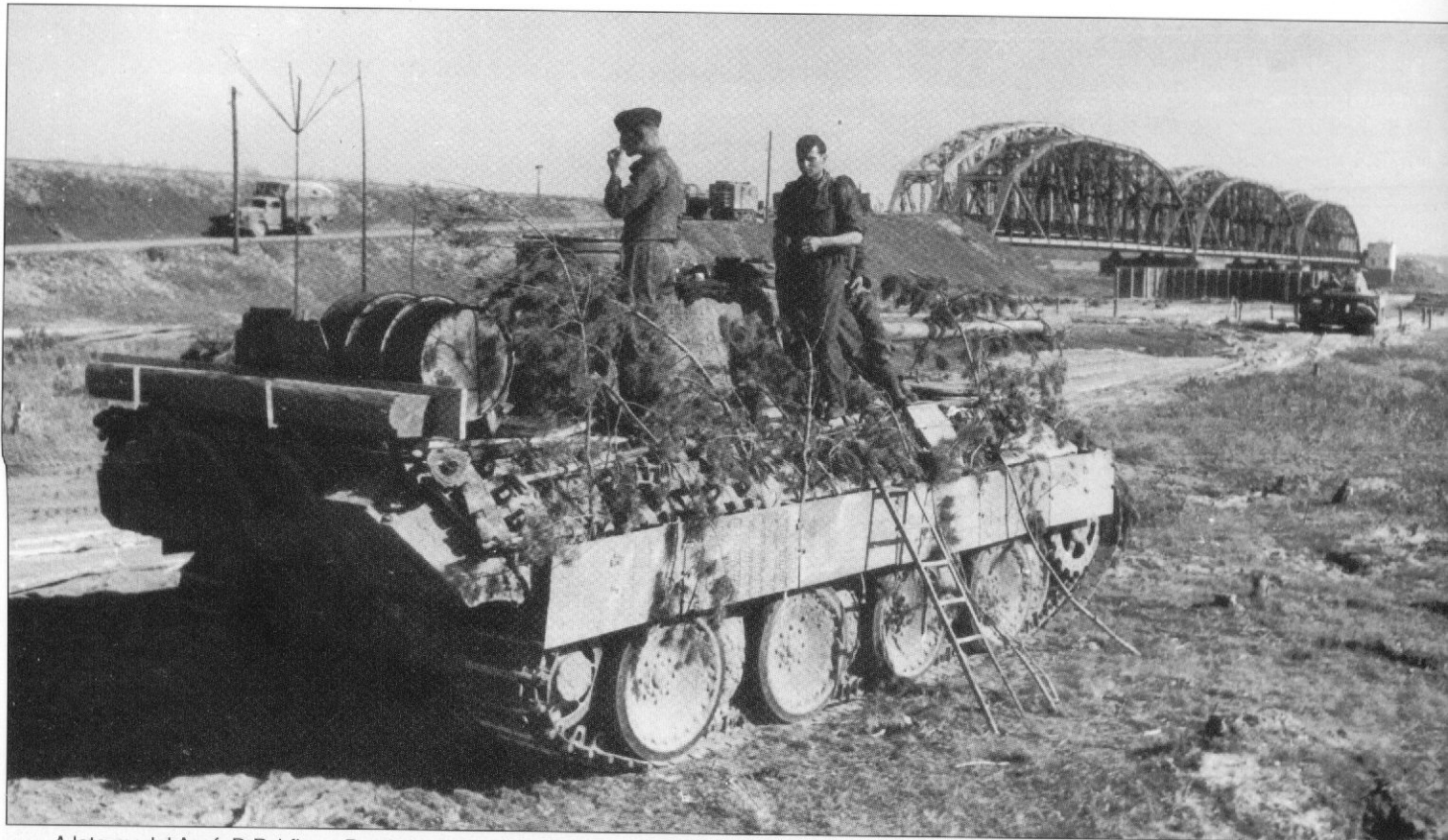
A late-model Ausf. D Pzbfswg Panther supervises a railway bridge. This particular tank is interesting because it shows the 6-ft (2-m) rod antenna fitted to the left mount on the hull rather than to the turret's antenna mount, making it clear that any configuration was possible. A lot of extra equipment was carried on the engine deck. (W. Schneider)
