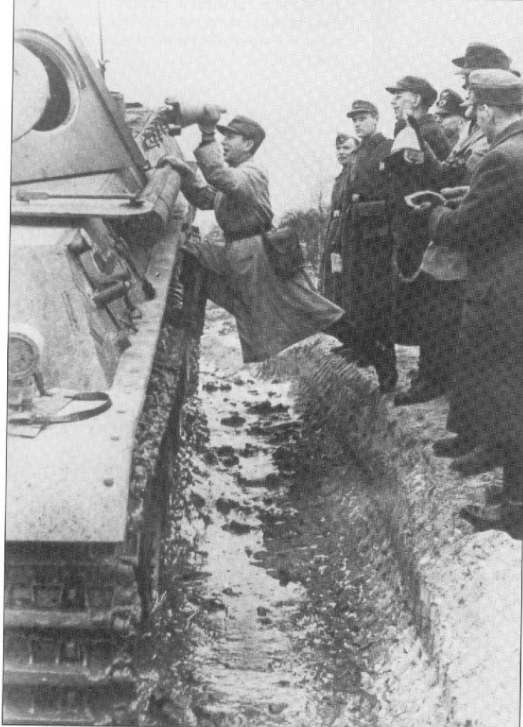
This undamaged Panther was abandoned at Tisnov, Czechoslovakia, at the end of April 1945. This is a very late Ausf. G fitted with a flame suppressor exhaust. A lot of extra equipment is carried on the engine deck and the turret. (S. Netrebenko)
