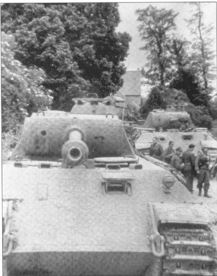
Tanks of 5.SS-Pz.Div. "Wiking" prior to combat near Kovel in April/May 1944. This unit played an important part in breaking through the pocket around that city. Both vehicles, late Ausf. Ds, show partly damaged Zimmerit coatings. The camouflage consisted of narrow stripes of dark green and brown over the dark yellow base, which were probably applied with brushes. The Panther at right shows a 6.5-ft (2 m) rod antenna fitted on its roof and a 4.5-ft (1.4 m) rod antenna on the standard mount behind the turret. That means this could be a Flivo tank (Sd.Kfz. 268 ground-to-air liaison vehicle). (W. Schneider)
