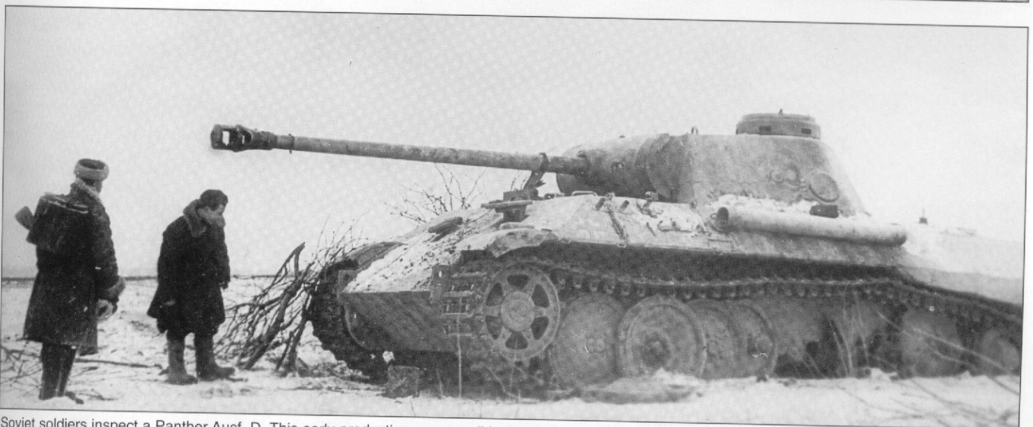
Panther "428" was painted over with whitewash. The large numbers on the side of the turret and the smaller one at the rear were painted very crudely in red. An iron cross is visible between the exhaust tubes. The Zimmerit was probably applied by a field workshop. Note that both track tension ports are opened, and the tension tool is still fitted in the left one. (S. Netrobenko)
