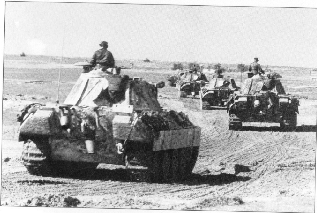
A platoon of Panther Ausf. As of "Wiking" moves to the front. The Panther in the foreground is fitted with ventilation pipes at the left exhaust. The jack is fitted between the exhaust tubes. Note the loader sitting in the rear hatch. (W. Schneider)
