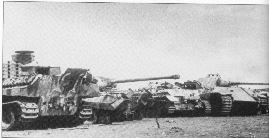
A similar vehicle lies in a heap near a railroad track somewhere in eastern Germany. Note the late-style flame suppressor exhaust tube. Brackets were welded on both sides of the turret to carry extra road wheels. (S. Netrebenko)
