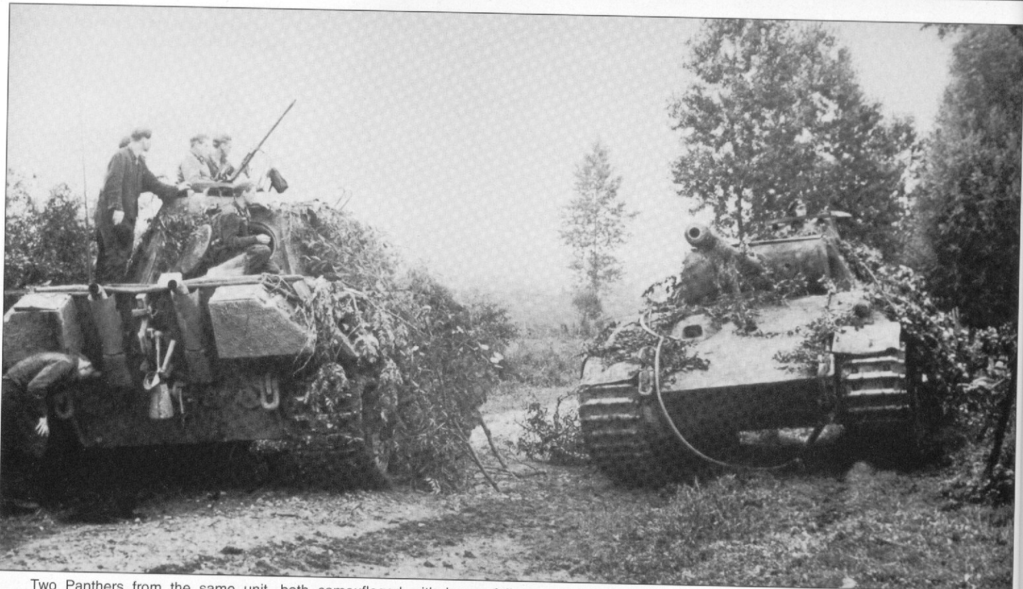
Two Panthers from the same unit, both camouflaged with heavy foliage, meet on a road. The Panther on the left carries an MG 34 in a Fliegerbeschussgerät (AA mount), but the ammunition drum is not fitted. The exhaust has been provided with protective covers, and the jack is mounted between the pipes. A towing rope (which would probably be lost soon) has been very slovenly attached to the Panther at right. (F. Schulz)
