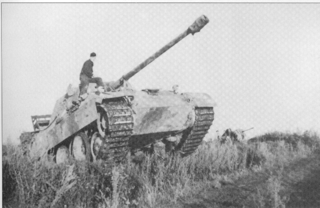
Panther "632" negotiates a slope. These situations could become serious, as the bottom of the tank featured only weak armor. Additionally, enemy shells would hit the plates at 0 degrees, making penetration very likely. This tank was converted to a mobile veranda by adding what looks to be quite a comfortable bench. (K. Münch)
