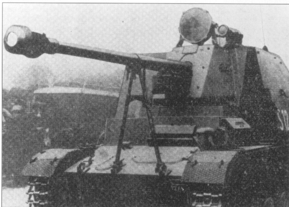
IR night-vision equipment was tested on many different vehicles. This Marder II, wearing the number “S 12”, shows an IR search light/image converter combination on top of the Pak 40. Another image converter was added to the left of the driver's side visor. (F. Schmidt)
