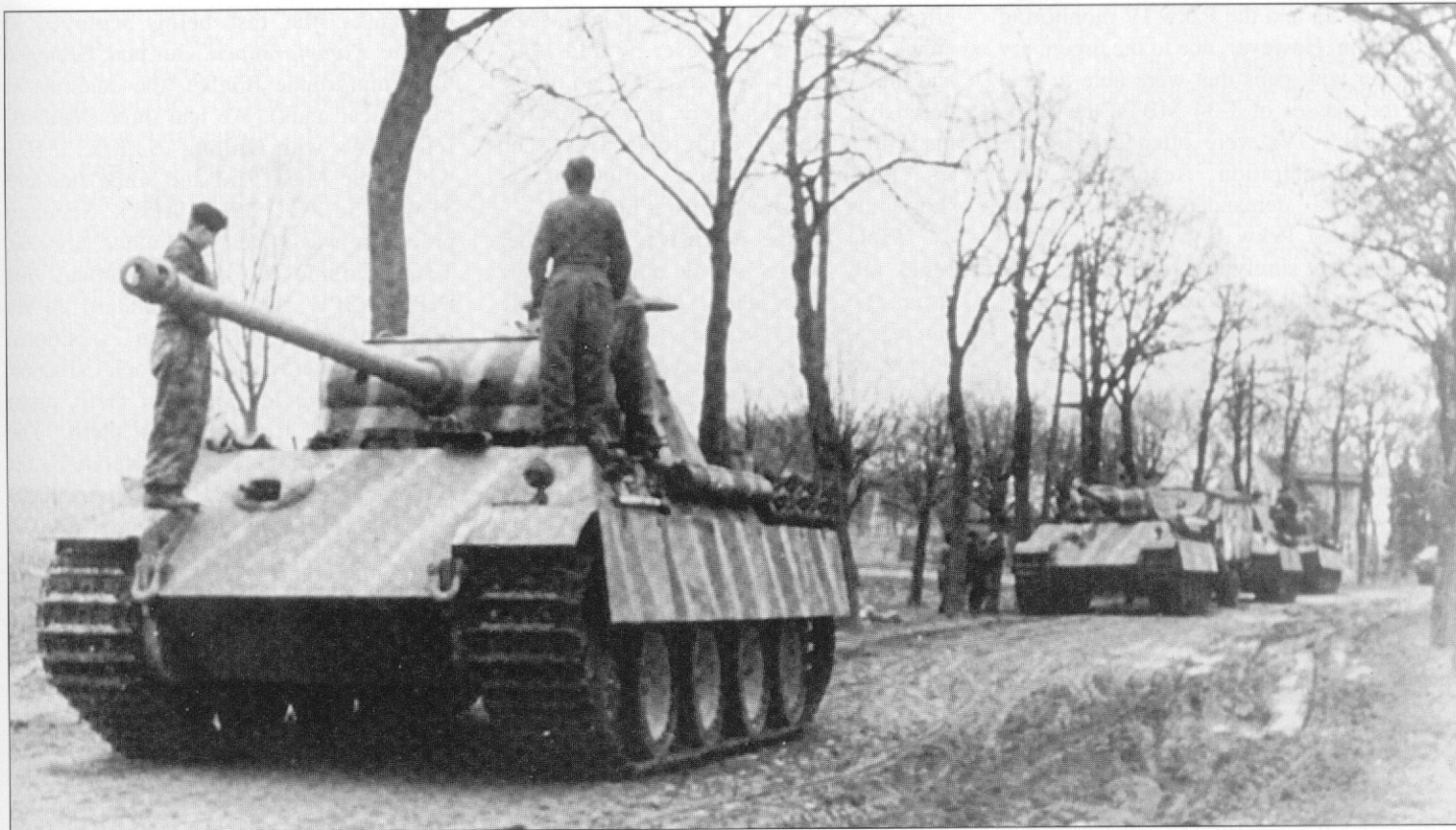
Photographed in February 1945, these late-model Panther Ausf. Gs move into defensive positions at the village of Ortwig near Küstrin. Here the Soviets had built up a bridgehead some 31 miles (50 km) east of Berlin. The Panthers show the distinctive reinforced gun mantlet. For camouflage, diagonal stripes were sprayed in broad lines over the dark yellow base color. (BA)
