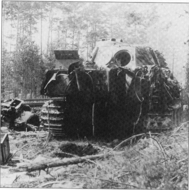
The blast of an internal explosion blew the turret off of this Panther Ausf. G. Of interest is the unusual turret number, "A J 9", the meaning of which is unknown. (S. Netrebenko)
