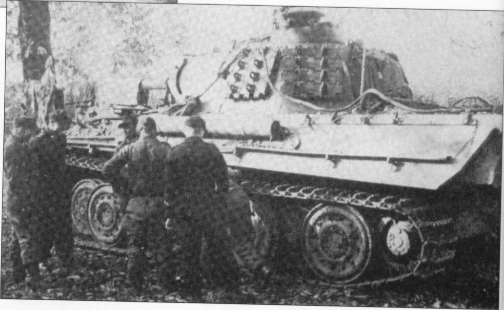
Back from combat near Aachen. This interesting photo shows a Panther Ausf. G of Pz.Rgt. 24 with steel-rimmed running wheels. An O-series was provided with these rubber-saving wheels, probably due to the good experiences the Tiger tanks had with them. This tank also shows a lot of extra equipment. Note how blankets have been hung out to dry from the gun barrel. (E. Bernhardt)
