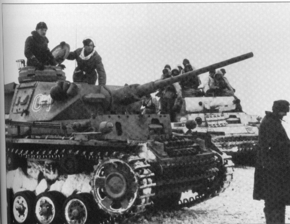
The Pzbfswg III Ausf. K was the first command tank to be provided with a standard tank gun. The 50 mm L/60 was shifted to the left, thus creating space for additional radio equipment in the turret. These vehicles carried a less conspicuous star antenna instead of the frame antenna. (F. Schulz)
