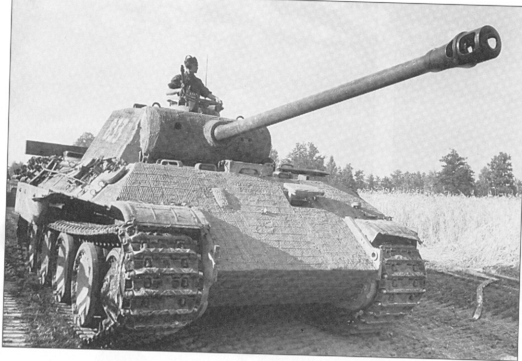
This photo shows the impressive sight of the Panther MBT. This late Ausf. D (binocular gun sight) is covered with a factory-applied Zimmerit coating. The turret number "833", was handpainted in white. Note that the front sections of the side skirts and parts of the mudguards are missing. (W. Schneider)
