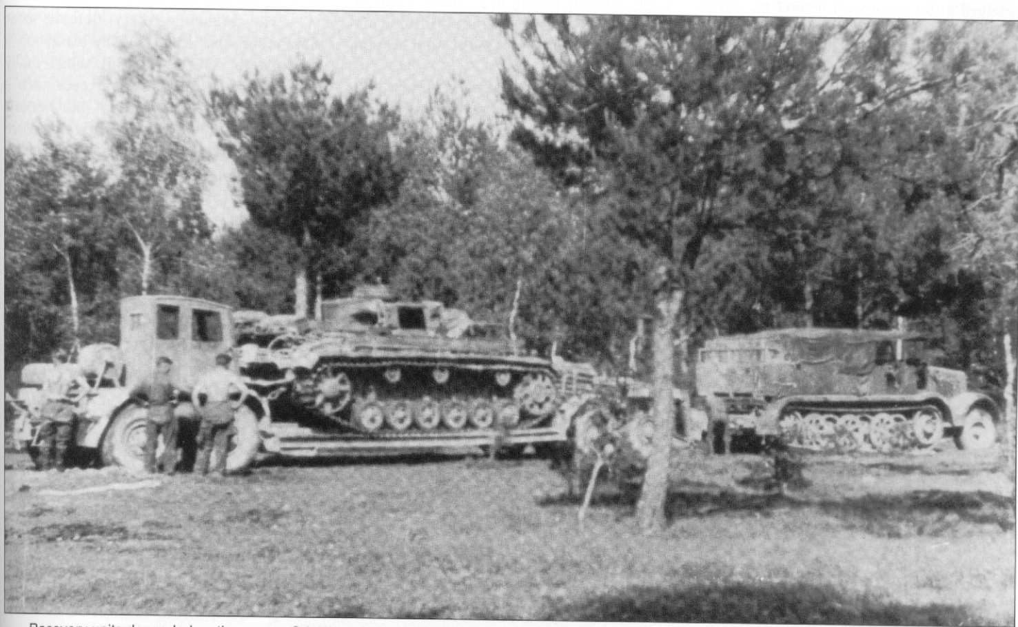
Recovery units depended on the proven Sd. Kfz. 9 heavy half-track and the Sd.Anh. 116 trailer. This combination was sufficient when dealing with Pzkw IIIs or IVs that weighed up to 20 tons. This particular flatbed trailer, which is being towed by a 12-ton half-track, is interesting since it shows a fully closed rear steering cabin. (W. Schneider)
