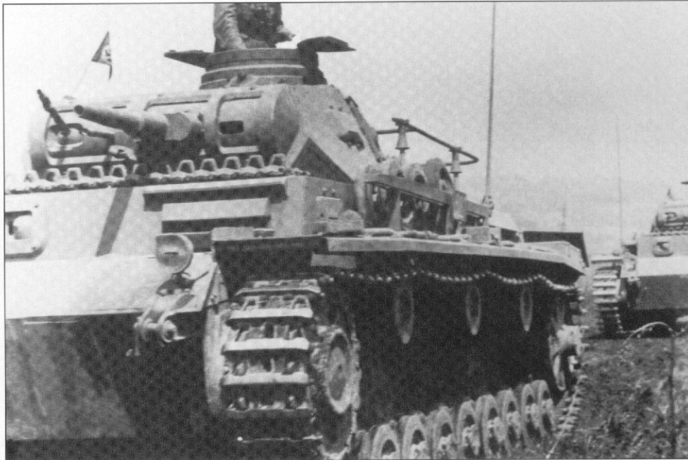
The high degree of communication was one reason for the success of German armored forces. Command tanks like this Pzbfswg III Ausf. B provided the troops with reliable long-distance radio systems. The early command tanks featured dummy guns and highly conspicuous frame antennas. (BL)
