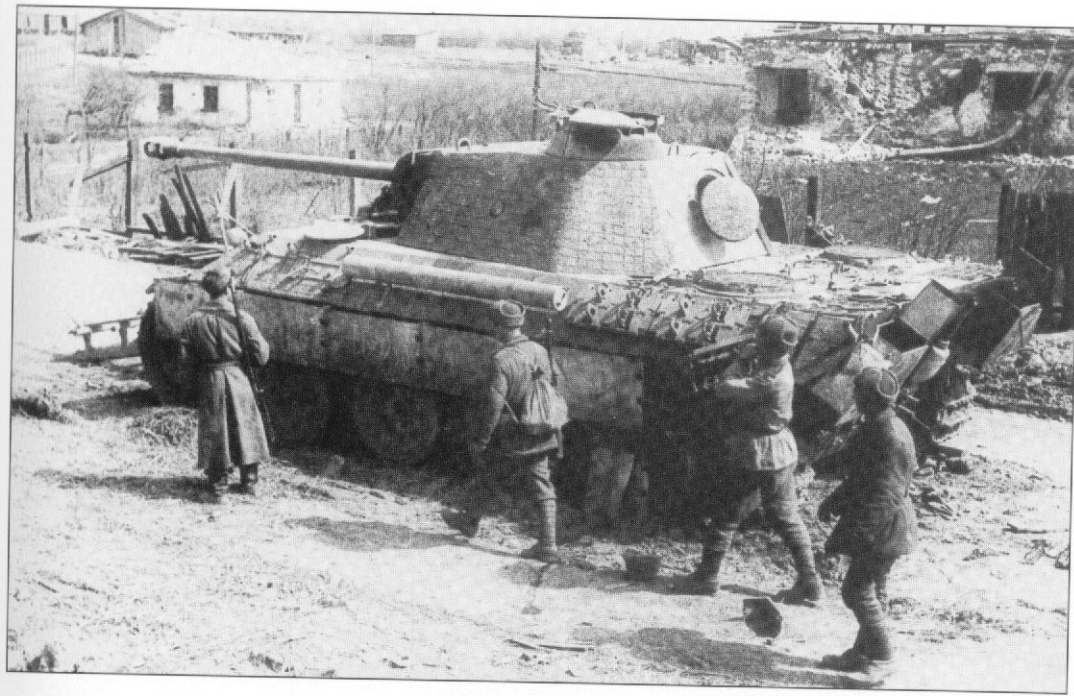
A Soviet infantry squad passes by a destroyed Panther Ausf. D (late production). Both the communication port and the smoke grenade dischargers were deleted during production. The tank is fitted with the later cast commander's cupola. Since all hatches are open, the crew probably managed to escape. (S. Netrobenko)
