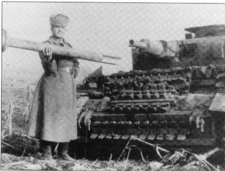
This Pzbeobwg III Ausf. H was heavily converted to be integrated in Pzkw IV units. The original dummy gun was converted with a longer wooden beam and a muzzle brake so the tank would resemble the 75 mm KWK-armed Pzkw IV. Zimmerit and a full set of side skirts were added in a field workshop. This photo was taken in Kursk in the summer 1943. (S. Netrobenko)
