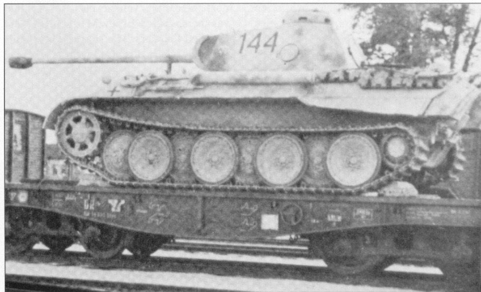
This obscure photo shows a Panther of Pz.Abt. 52 during Operation "Zitadelle". Since the power train was prone to breakdown, every opportunity was used to entrain Panther units. Note that the smoke grenade dischargers have been removed. The tanks of Pz.Abt. 52 display a roaring Panther's head as an unofficial unit badge. (M. Green)
