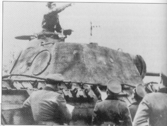
A late-model Ausf. D Pzbfswg Panther supervises a railway bridge. This particular tank is interesting because it shows the 6-ft (2-m) rod antenna fitted to the left mount on the hull rather than to the turret's antenna mount, making it clear that any configuration was possible. A lot of extra equipment was carried on the engine deck. (W. Schneider)
