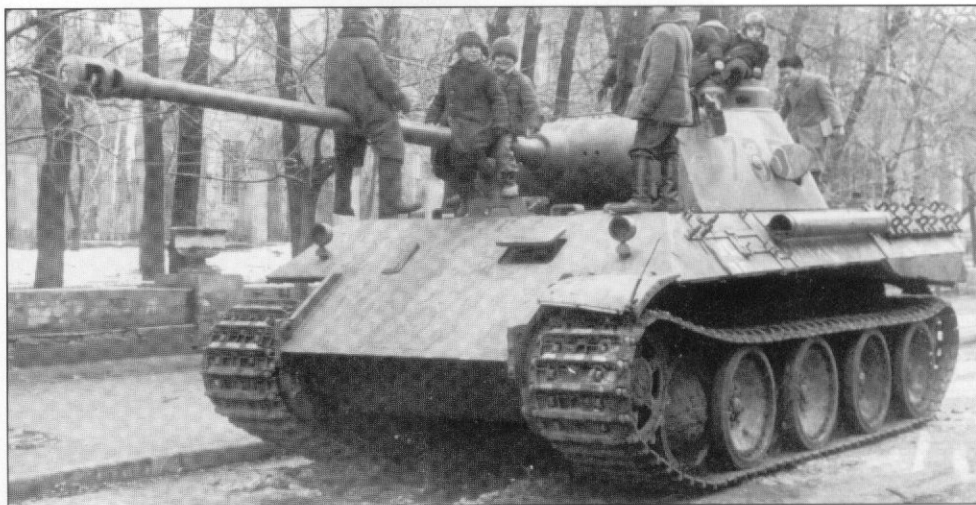
Russian children playing on an abandoned Panther Ausf.D of Pz.Abt. 52. Number "735" is in excellent condition, proving that it was lost to minor damage. The driver's visor is half opened. Although this hatch provided the driver with a good view, it weakened the front armor protection. Note that the reloading/communication hatch is also open. (S. Netebenko)
