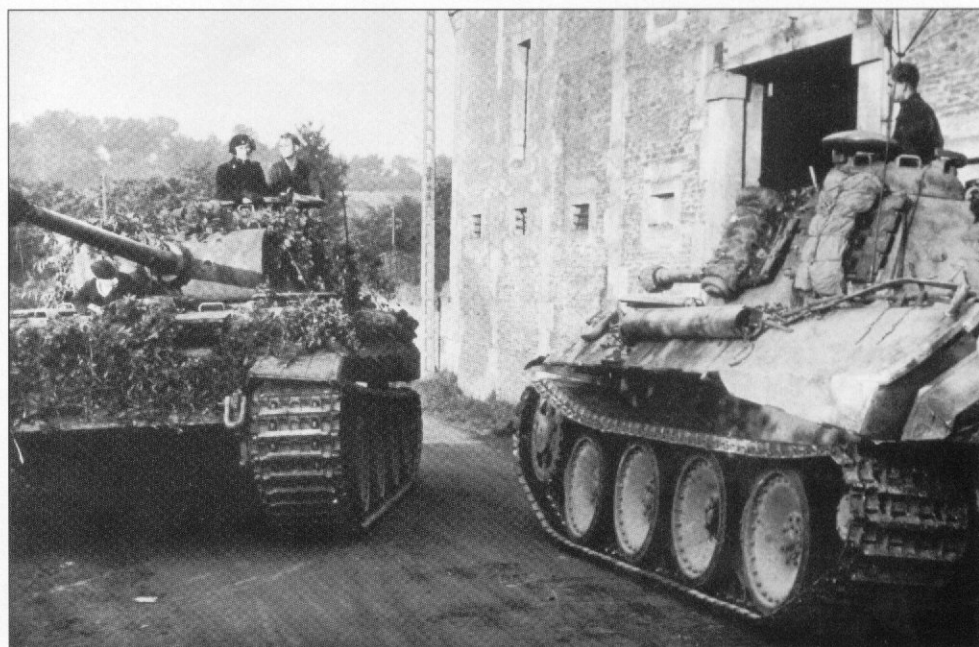
The same vehicle from behind. The "incorrect" position of the star antenna is evident here. The three elongation tubes for the star antenna, which are normally stored below the gun cleaning kit, are missing. (F.Schulz)
