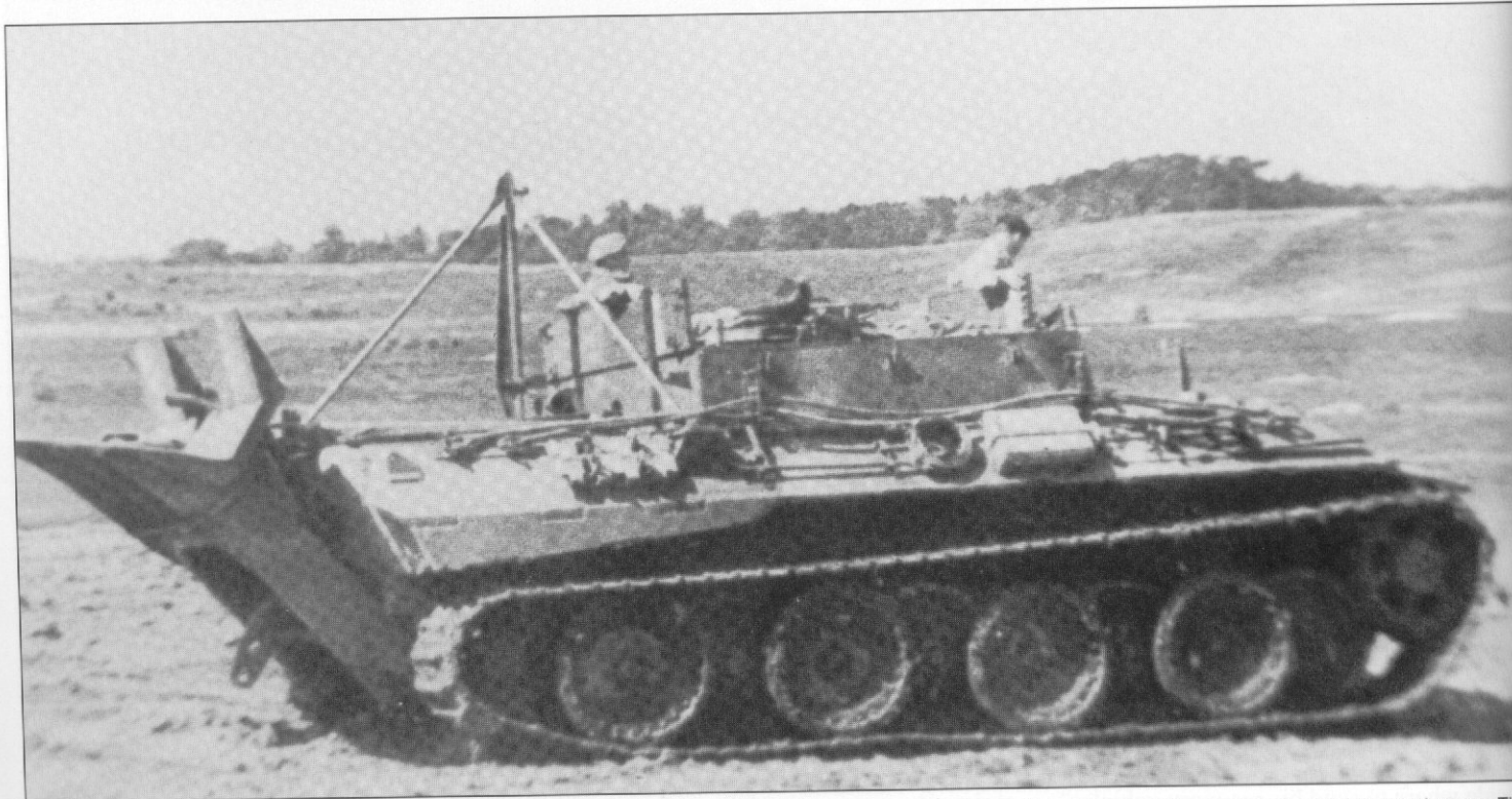
The British soldiers seen here can't help but be impressed as they evaluate this Bergepanther, which shows off its rear spade and erected crane. The latter could be mounted on either side of the engine deck. A lot of recovery equipment is visible in this photo. (A. Geibel)
