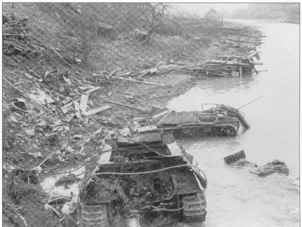
This photo shows the result of an Allied air strike that surprised a unit while it was crossing a bridge. The Bergepanther is totally destroyed, providing us a view into the engine and winch compartment. (J. Mueller)
