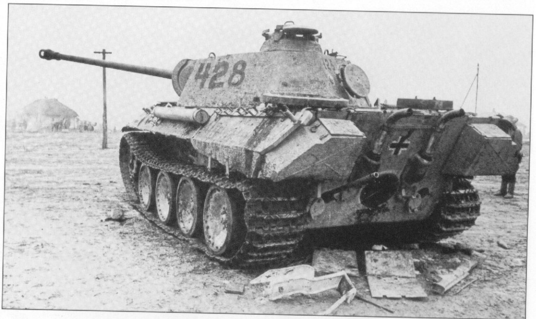
Panther "428" was painted over with whitewash. The large numbers on the side of the turret and the smaller one at the rear were painted very crudely in red. An iron cross is visible between the exhaust tubes. The Zimmerit was probably applied by a field workshop. Note that both track tension ports are opened, and the tension tool is still fitted in the left one. (S. Netrobenko)
