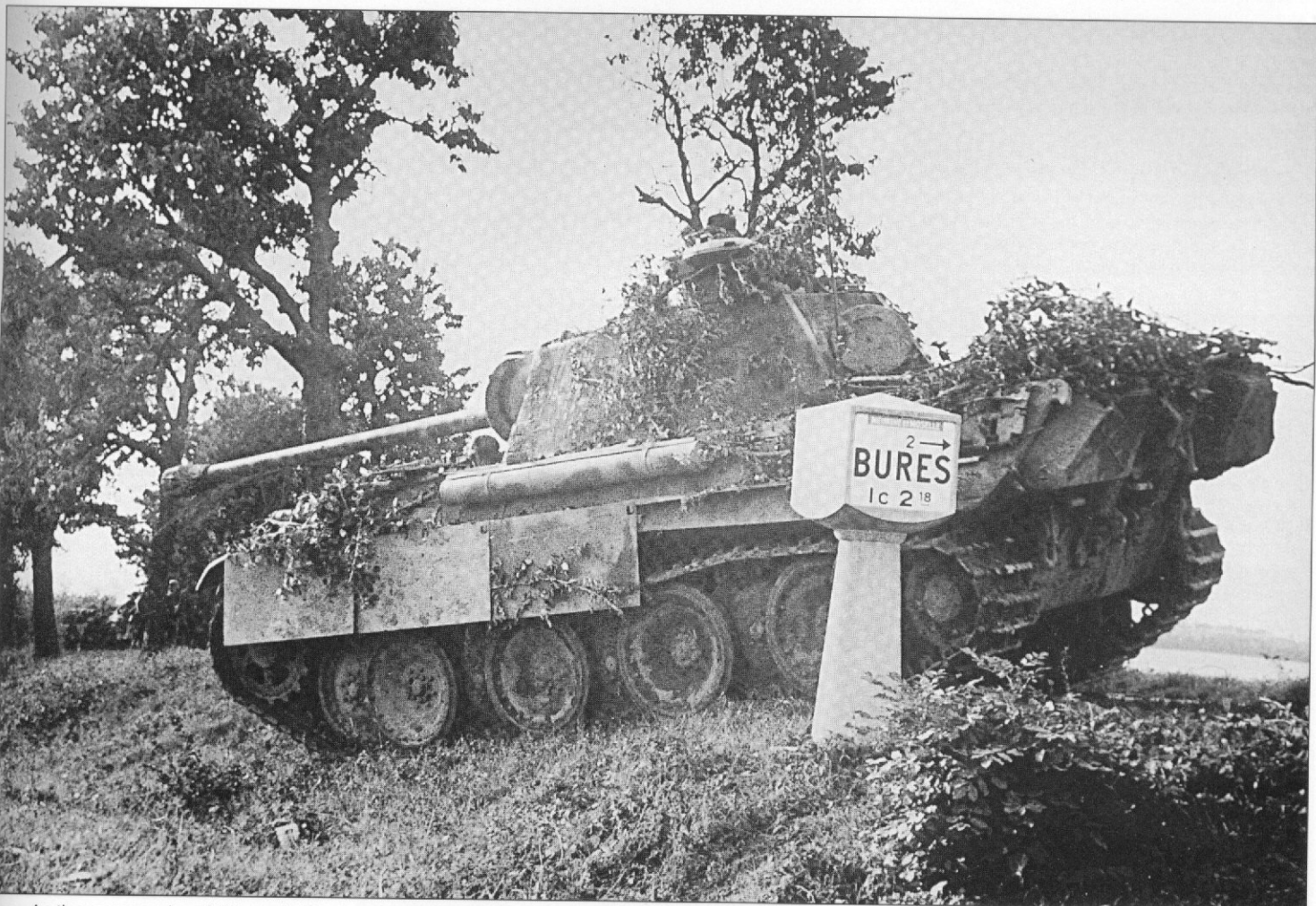
As the commander of this early Panther Ausf. G scans the terrain carefully from his cupola, he steers the tank off the road to search for cover in the shadow of some trees. The tank's last two side skirts are missing (something that happened rather often). The rear hatch was held open for better ventilation. (F. Schulz)
