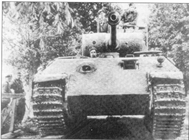
This Ausf. A, photographed in Italy, shows an unusually scruffy Zimmerit coating that was slovenly smeared over the vehicle without any rippled pattern being created. Note the ice cleats on the tracks. The gun sight is of the later monocular type. (W. Trojca)
