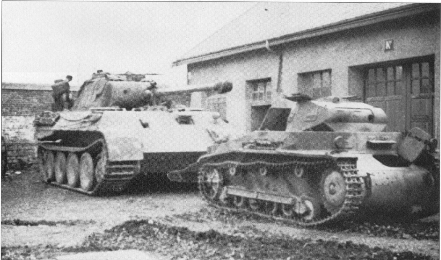
The same vehicle from a distance. In front of it an archaic vehicle, a Pzkw II Ausf. B, can be seen. Oldtimers like this were used for tank school driving purposes up to the end of the war. The tanks of Pz.Rgt. 24 received their Zimmerit coating at field workshops in September/October 1943, resulting in a scruffy and uneven pattern. (E. Bernhardt)
