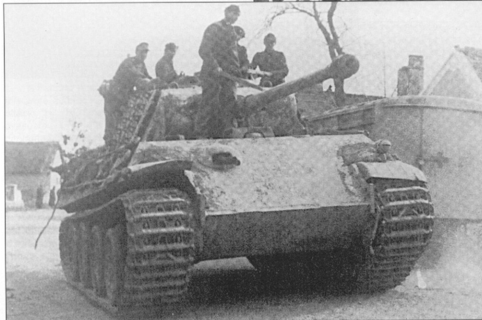
A Panther waiting for action in a French town. The hatch on the driver's side was deleted with the advent of the Ausf. G. The vehicle lacks all side skirts but carries extra track links for additional turret protection. (P. Kammann)
