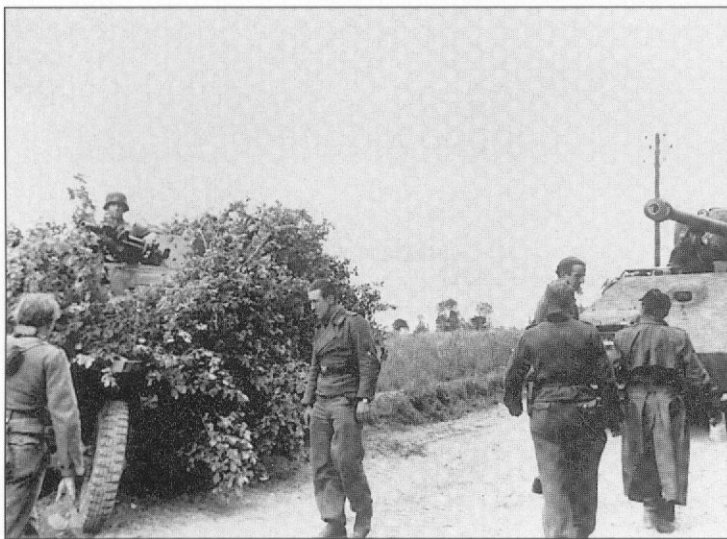
This bush is an APC! The crew of the Sd.Kfz. 250/10 (yes, this is evident by the wheels) did a good job of concealing their vehicle. The only visible crew member holds his hand on the 37 mm Pak 36. (F. Schulz)
