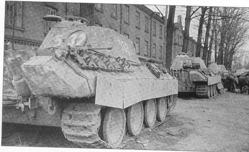
Panthers of 5. Company (probably of "Wiking") assembled at a factory yard. The first vehicle, which is probably an Ausf. D, illustrates the original horizontal position of the jack. The next Panther is an Ausf. A, as is evident by the vertical jack and the cooling pipes attached to the left exhaust. The tanks display a very scruffy camouflage of dark brown and dark green stripes. Covered in mud and dust as all of them are, the tanks blend in perfectly with their surroundings. (W. Schneider)
