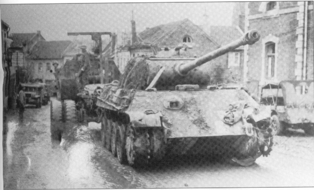
Destroyed on the Western Front, this Panther Ausf. G is being hauled by a M25 Dragon Wagon. Note how large portions of the Zimmerit coating have fallen off. (A. Geibel)
