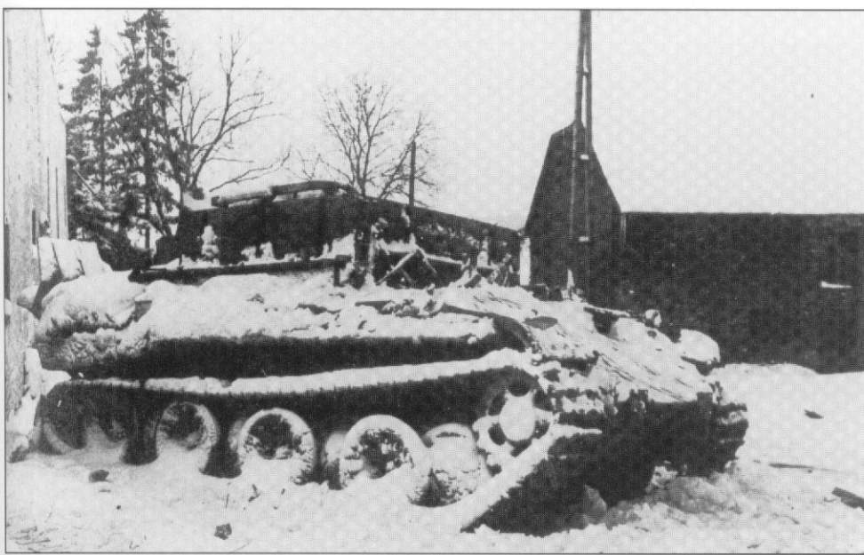
A Bergepanther Ausf. D lies abandoned in a French town. The wooden body was large enough to carry replacement engines or transmissions, which could be fitted using the crane. (J. Mueller)
