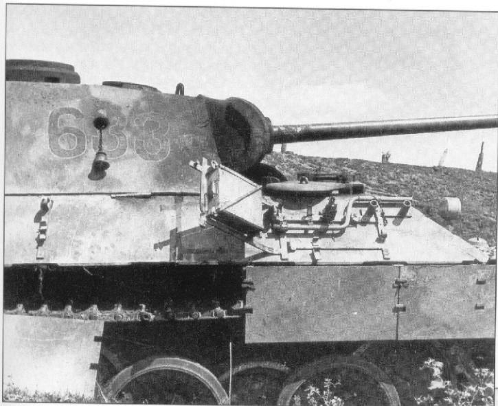
Panther number "633", an early Ausf. D of Pz.Abt. 52, was destroyed during Operation "Zitadelle". Note the pistol port cover hanging at its chain, which was possibly blown out by an internal explosion. Also, the armor skirt supports are visible. This arrangement was quite prone to damage, and many Panthers lost their skirts during combat. The crews often fixed additional brackets for them. A Panther head insignia is barely visible in front of the turret number. (S. Netrebenko)
