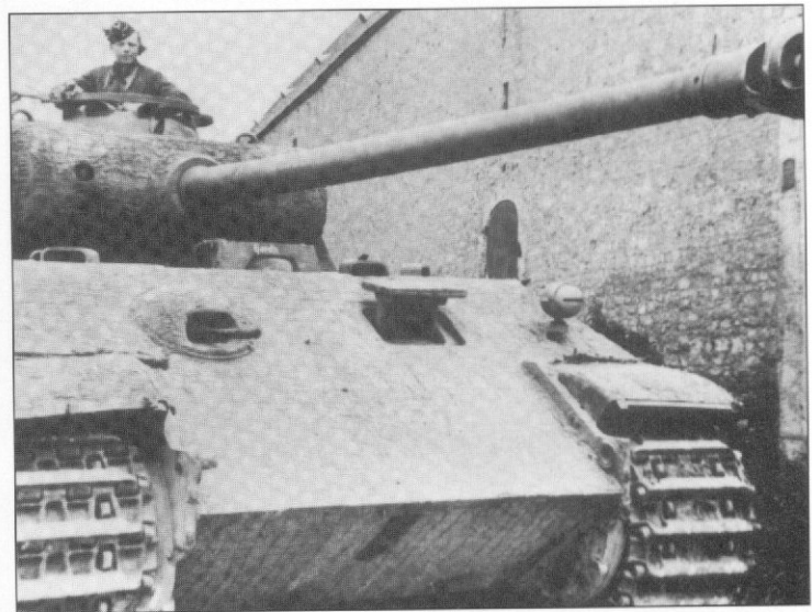
This Ausf. A Panther offers a good view on its factory-applied Zimmerit . Note that the gun's travel rest is folded away, and the name "Gerda" is written on the mount. (F. Schulz)
