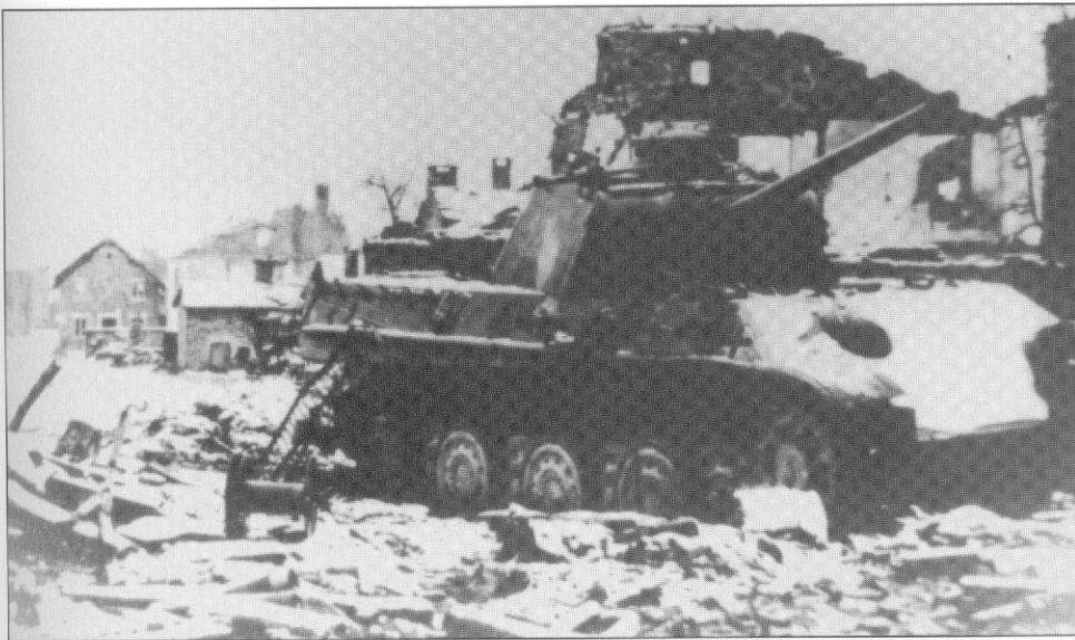
Another destroyed Panther Ausf. G with steel-rimmed running wheels. This tank probably became a victim of concentrated artillery fire. (E. Bernhardt)
