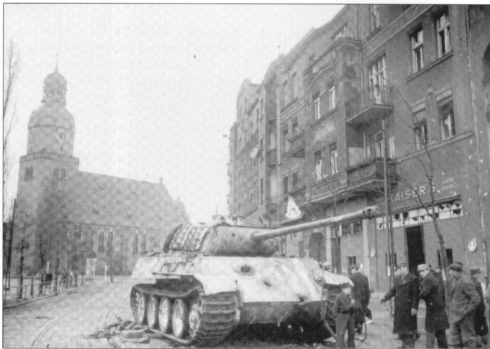
This Panther Ausf. G was destroyed in the town of Posen. It shows two penetrations at the hull front, probably from an 85 mm gun. Both shots were probably stopped by the transmission, allowing the crew to escape. As typical for late-war Panthers, the vehicle carries extra tracks and spare running wheels on the turret. The tank has been camouflaged with whitewash. (S. Netebenko)
