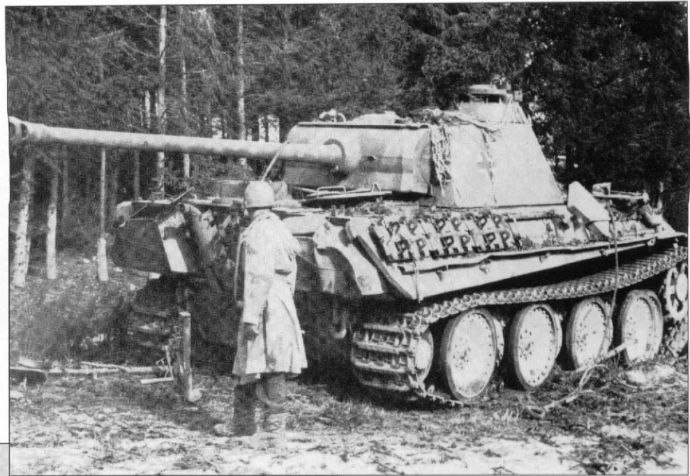
The chin-type gun mantlet prevented shells from being deflected to the thin roof, thus improving the level of ballistic protection. This late Ausf. G was provided with the raised engine cooler on the left side, and its exhaust pipes are fitted with protective covers. The German cross on the turret was non-standard. Overall, Panther "302" seems to be undamaged. (M. Green)
