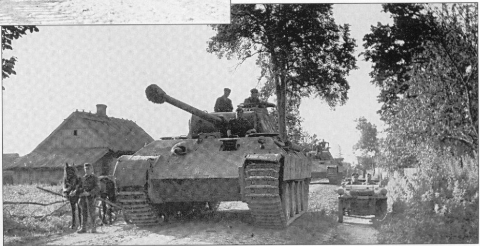
This Ausf. A of "Wiking's" 8. Company (2nd Battalion) also features a glacis plate that is devoid of Zimmerit . (Perhaps small arms fire shot it away?) The passing VW Schwimmwagen provides a comparison by which we can get an impression of the large bulk of the Panther. (W. Schneider)
