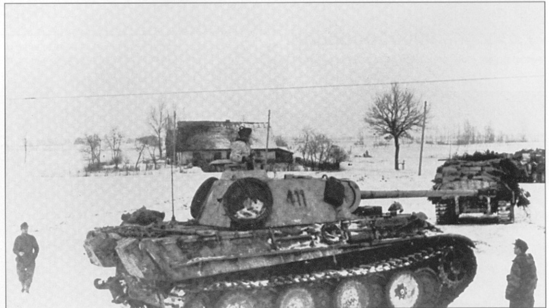
On the 15 January 1945, the Soviets launched a major assault on East Prussia. These Panthers are assembling for a counterattack. Winter whitewashed Panther "411" shows a lot of extra equipment, typical for the last months of the war. If the crews were resupplied, the vehicles would carry as much as they could hold. Two extra running wheels are fitted to the turret. In the background is visible a Bergepanther recovery vehicle. (BA)
