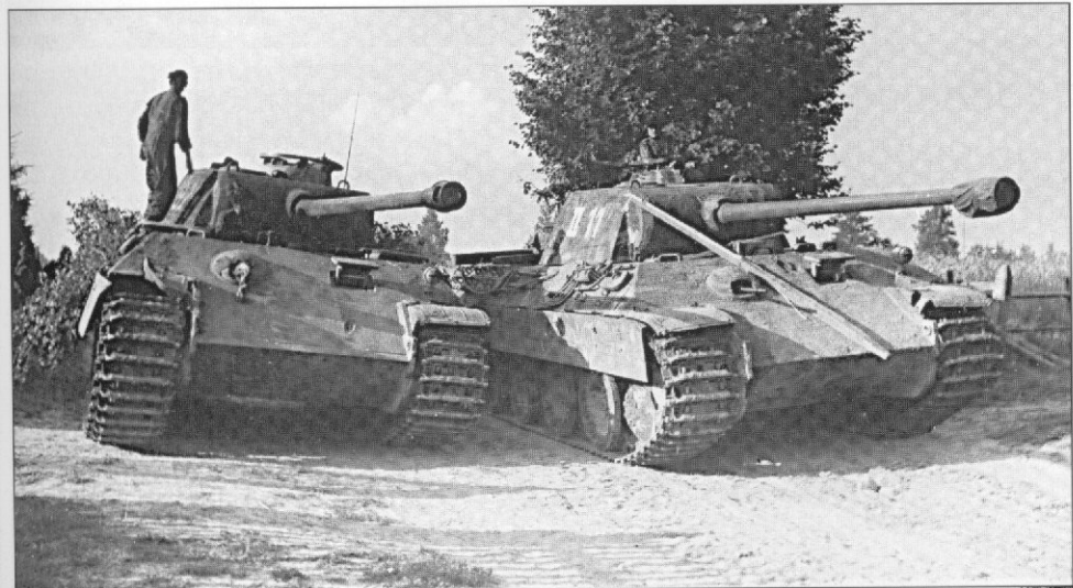
This Ausf. A of "Wiking's" 8. Company (2nd Battalion) also features a glacis plate that is devoid of Zimmerit . (Perhaps small arms fire shot it away?) The passing VW Schwimmwagen provides a comparison by which we can get an impression of the large bulk of the Panther. (W. Schneider)
