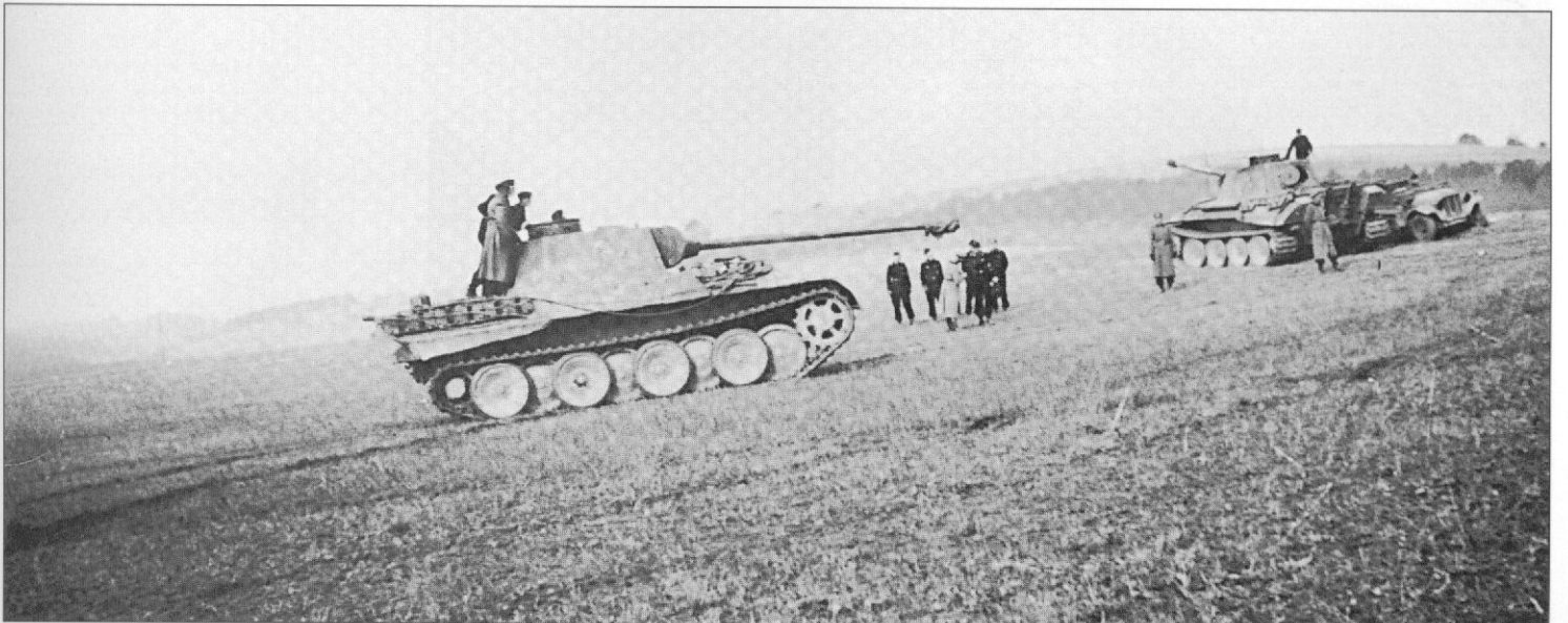
One-ton half-tracks provided the Panther tanks with new ammunition. Results of the live firing were discussed with officers of the 3rd Squadron. During training the Panthers had their side skirts removed to avoid unnecessary losses. (E. Bernhardt)
