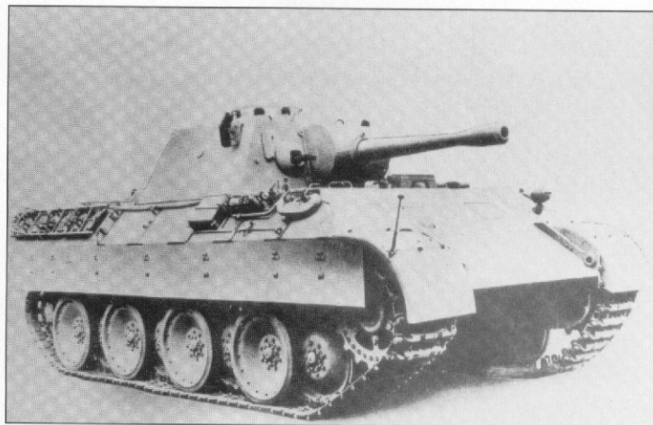
This is the only photo known to the author that shows the Pzbeobwg Panther. Based on a late-model Ausf. D, the tank's turret was heavily modified. A short dummy gun replaced the L/70 gun. The right flap of the rangefinder that was integrated into the turret front plate is visible beside the machine gun's ball mount. (A. Geibel)
