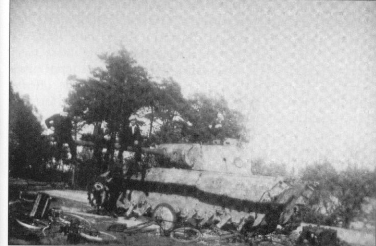
This crippled Panther lay near the town of Uelzen for a long time before it was fully scrapped. This early Ausf. D still shows two welding marks on the mantlet below the gun sight. It is possible that this vehicle was provided with a triple IR set of Solution B. (F. Schulz)
