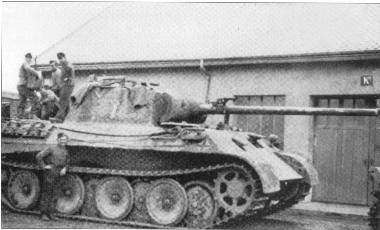
Pz.Rgt. 24 was established in 1943. After one year of hard fighting, it was sent to France for refitting. This photo was taken shortly after the invasion at a training area at Voussiers. This particular vehicle shows a mid-production Ausf. D. The commander's cupola shows an MG ring. The smoke grenade dischargers were already deleted. What makes this Panther interesting is the pyrotechnical gunfire simulator fitted onto the barrel just behind the travel rest. (E. Bernhardt)
