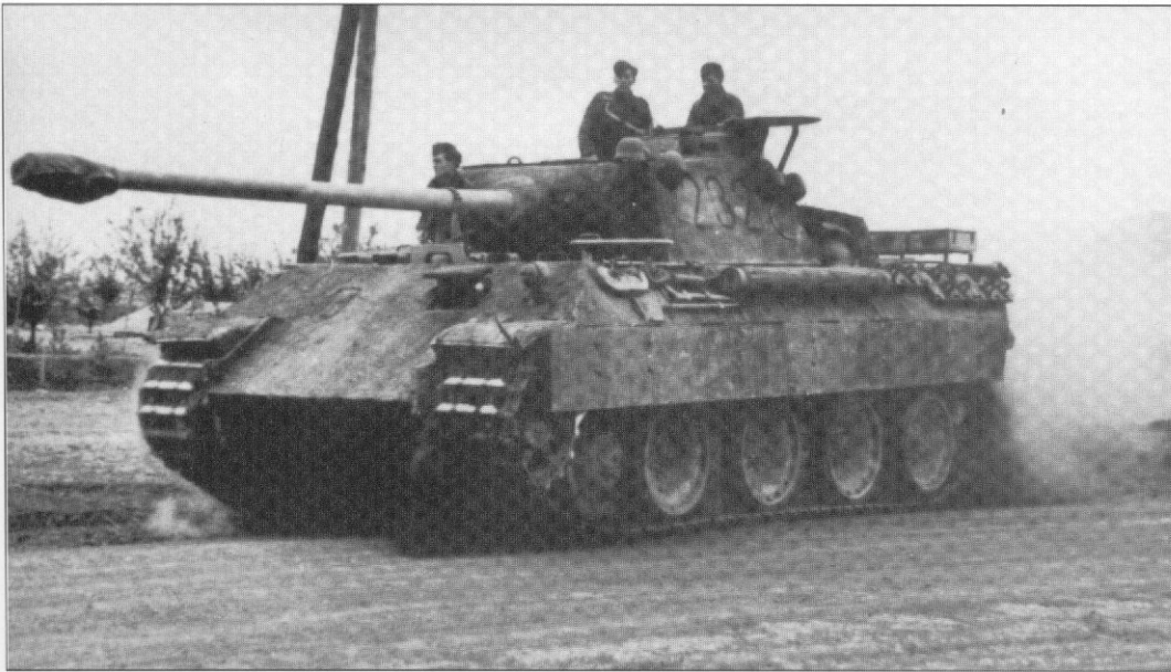
Panther number "232" is seen here speeding on its way. The crew has added a support for the swiveling commander's hatch. (The swivel hinge occasionally warped during rough driving.) Note that Zimmerit has even been applied to the side skirts. The crew's five steel helmets are stored outside the vehicle. (F. Schulz)
