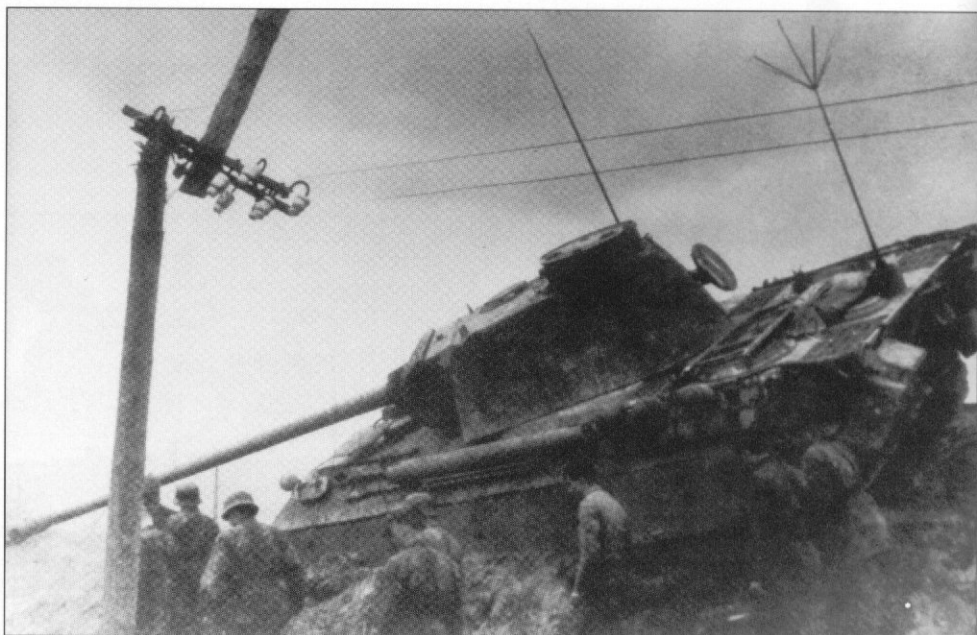
This abandoned Pzbfswg Panther Ausf. D, which has slipped off the rail line, features the standard equipment of a Sd.Kfz. 267: the 6-foot (2 m) antenna on top of the turret and the star antenna d in its armored pot located on the engine deck. The tank has also been provided with a ring for the AA MG. (P. Kammann)
