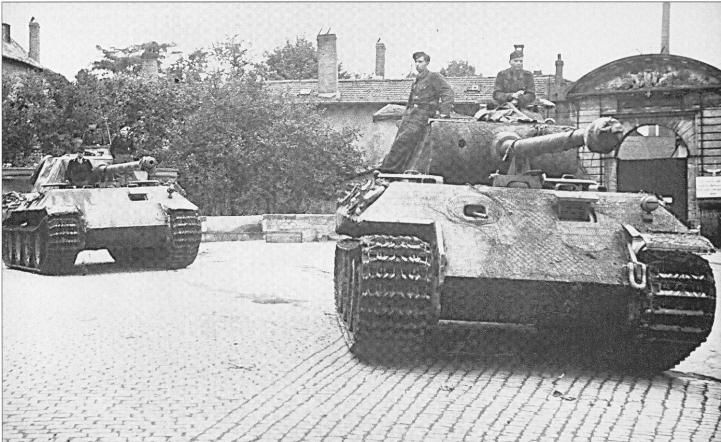
A late-model Panther Ausf. D follows an Ausf. A into a French town. The nearer vehicle is in marching order, its gun being fastened in the travel rest. A protective cover has also been pulled over the muzzle brake. (F. Schulz)
