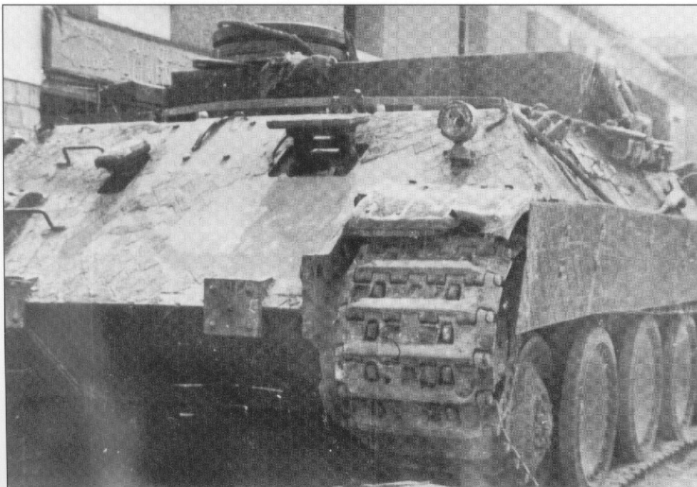
Another abandoned Bergepanther somewhere in France. Like most of these vehicles that we've seen, this is an Ausf. D. Both the driver's sight flap and the MG port are opened. Large portions of the Zimmerit coating have fallen off, possibly due to small arms fire. The wooden body is missing, and some extra roadwheels are visible on the metal superstructure. The 2 cm KWK mount was not fitted. (K. Münch)
