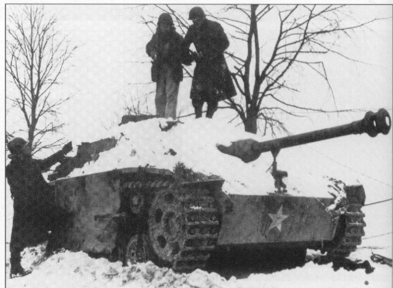
G.I.s inspect another concealed Stug III. This was a late-production vehicle, as the cast mantlet and the return rollers indicate. Pz.Brig. 150 conducted a number of unsuccessful assaults due to incorrect combat tactics. (J. Mueller)
