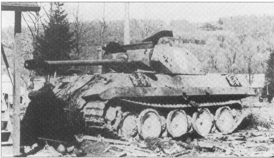
This Ersatz M10 was hit several times. The thin sheet metal has been partially ripped off by the impact of fire. (J. Mueller)
