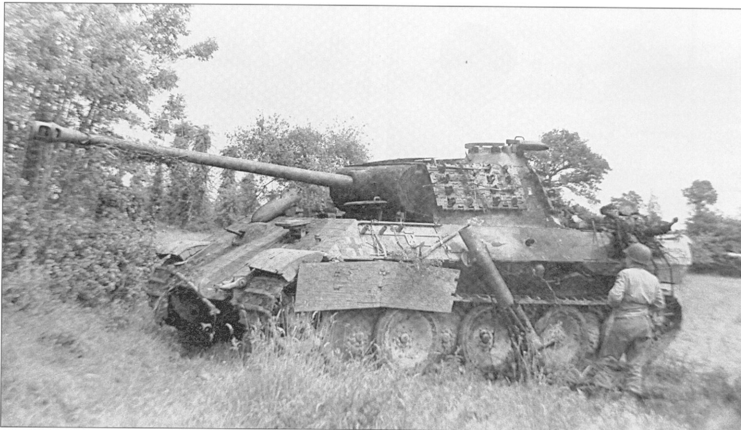
Destroyed by a round fired into its weak 1.7-inch (45 mm) side armor, this Panther lies abandoned in a French field. The turret's armor was reinforced by extra track links. (A. Geibel)
