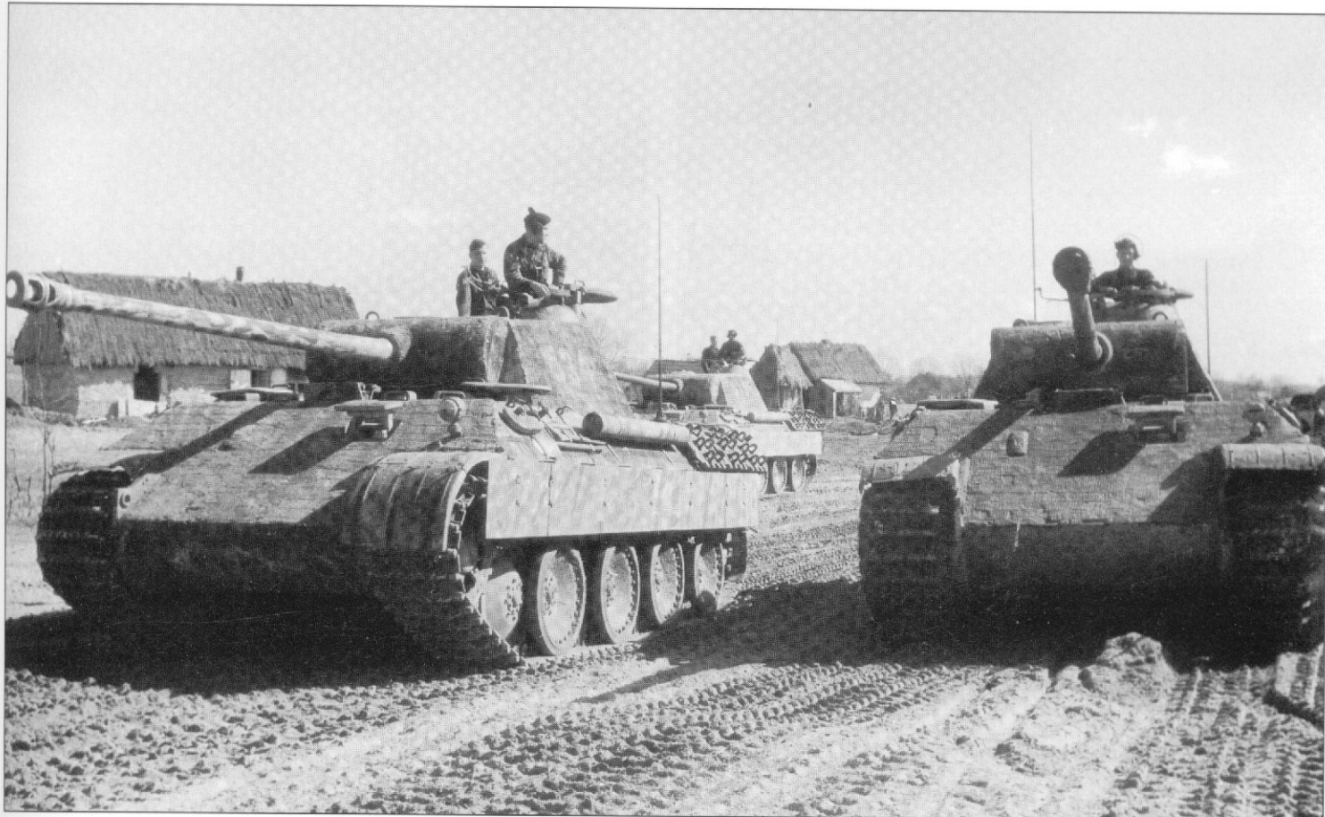
Tanks of 5.SS-Pz.Div. "Wiking" prior to combat near Kovel in April/May 1944. This unit played an important part in breaking through the pocket around that city. Both vehicles, late Ausf. Ds, show partly damaged Zimmerit coatings. The camouflage consisted of narrow stripes of dark green and brown over the dark yellow base, which were probably applied with brushes. The Panther at right shows a 6.5-ft (2 m) rod antenna fitted on its roof and a 4.5-ft (1.4 m) rod antenna on the standard mount behind the turret. That means this could be a Flivo tank (Sd.Kfz. 268 ground-to-air liaison vehicle). (W. Schneider)
